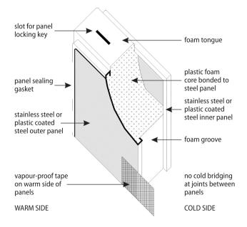
Generally the panel seal only needs to be continuous on the warm side. It is not necessary to seal the joints on the inside, because permeable joints on the cold side enable vapour to pass through and to condense on the evaporator plates. However, some argue that panels should be sealed on both sides, but that the sealant on the inner panel should be permeable.
