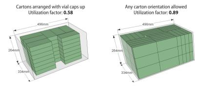
Many of these tools can handle the optimization of mixed loads – the most sophisticated versions are used to drive robotic pallet stackers.
